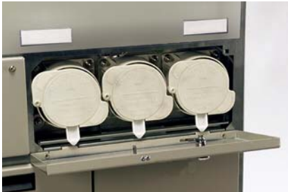
It is recommended that you replace all three fuses at the same time
