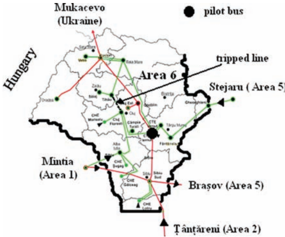
Figure 7.66. Area 6 interconnection lines with the neighboring areas and the tripped line in the test.
