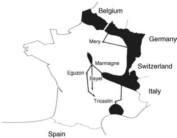
Figure 13.14. Part of the French grid still live at 8.26 a.m. on December 19, 1978 immediately after the first collapse [9].
