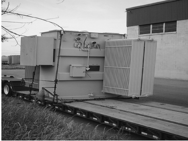
FIGURE 5.22 A 5000-kVA 18-pulse transformer ready for shipment. Motor drive duty, 13,800-V delta primary to secondaries of 1400-V delta, 1400-V delta +20°, and 1400-V delta -20°. (Photo courtesy of Niagara Transformer Corp.)
