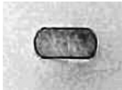
FIGURE 3.4 Cross section of enameled round wire after flattening. (By permission of ABB Inc., Jefferson City, MO.)
