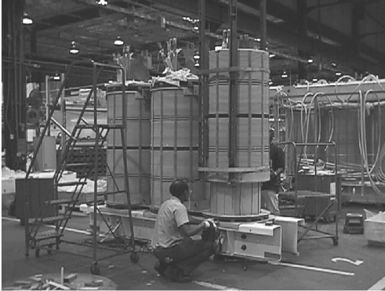
FIGURE 2.8 Concentric arrangement, outer coil being lowered onto core leg over top of inner coil.
