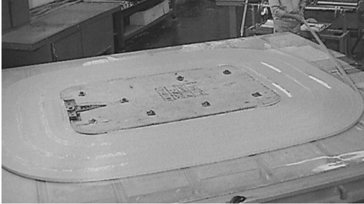
FIGURE 2.12 Pancake winding during winding process.
