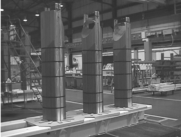
FIGURE 2.5 “E”-assembly, prior to addition of coils and insertion of top yoke.
