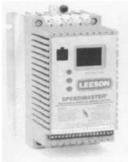
FIGURE 11 Low-power AC inverter (motor controller) for three phase motors with sine wave outputs and an output frequency range from 1 to 120 Hz (courtesy of Leeson Electric Corp.)
