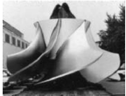
FIGURE 4 Mixed flow propeller runner (Voith Siemens Hydro)
