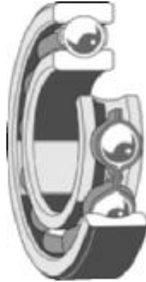
FIGURE 88 Single-row, deep-groove ball bearing (SKF USA, Inc.)
