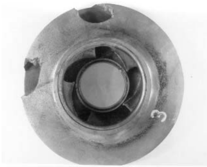
FIGURE 19 Overall view of a CF-3M impeller that has two corrosion-assisted fatigue fractures in the front shroud wall
