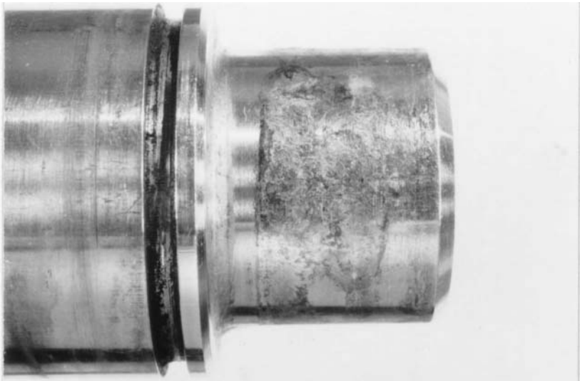
FIGURE 8 The fretting damage of a shaft beneath an impeller that experienced small amplitude motion. The mottled appearance is typical of the damage caused by fretting (2.2 \times ).
