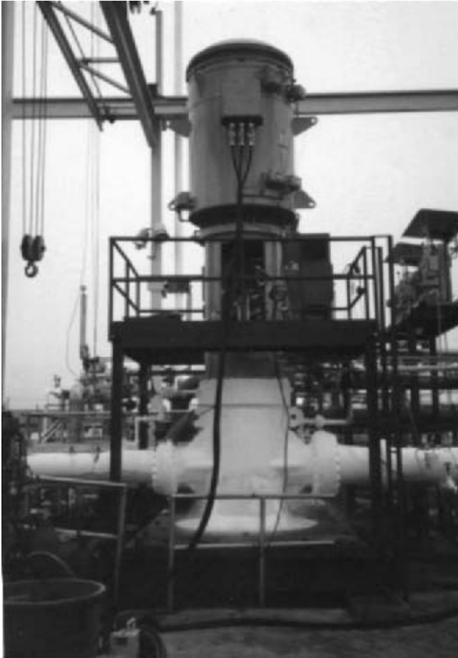
FIGURE 8 Multistage variable geometry expander on test stand (Flowserve Corporation)
