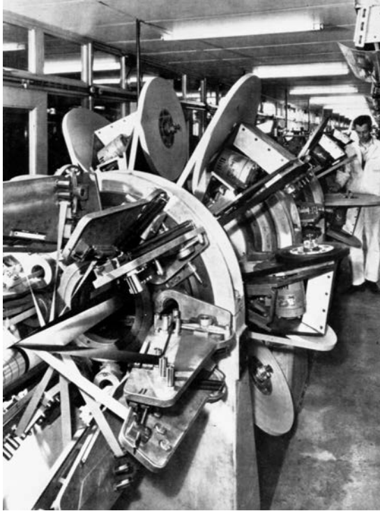
Figure 6.5 A lapping machine for applying paper insulation tapes
