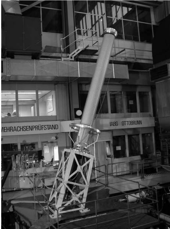
Figure 12.20 Seismic withstand test on polymer transformer bushing
