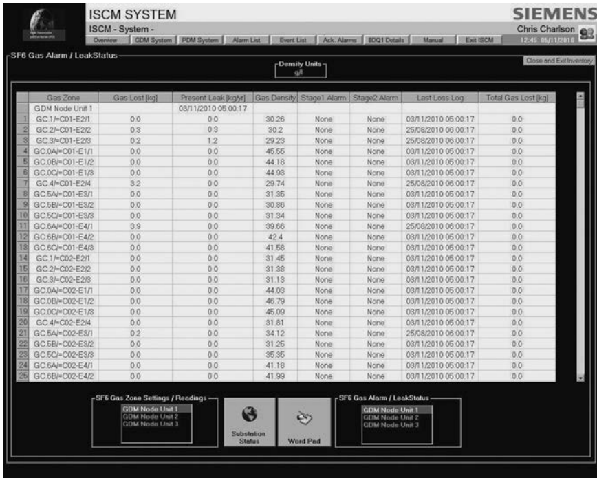
Figure 21.37 Gas density inventory screen
