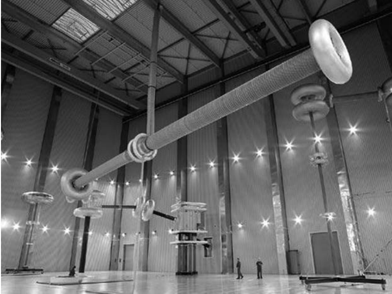
Figure 12.19 Bushing tests at HSP Laboratory, Cologne
