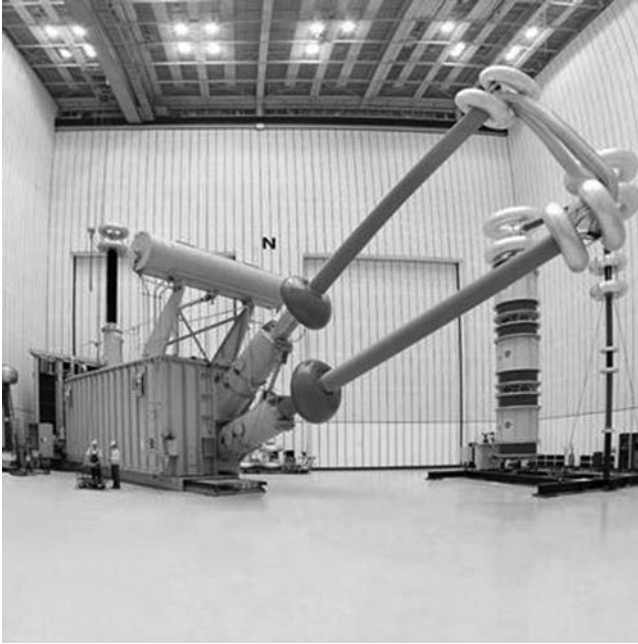
Figure 12.18 800 kV DC resin-impregnated paper bushings
