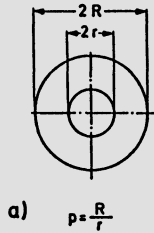
Fig. 1.1-6 Coaxial cylinder electrodes a) arrangement b) utilization factor
