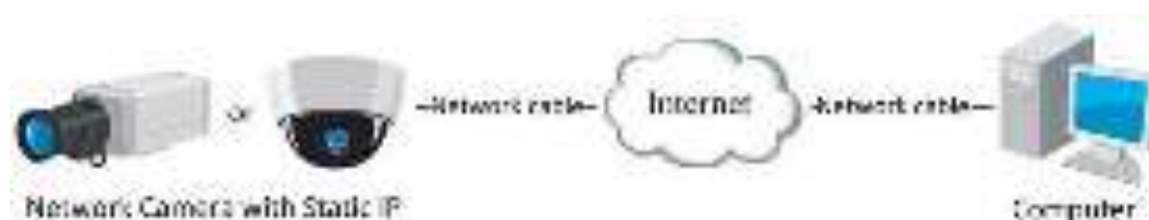
Figure 2-11 Accessing the Camera with Static IP Directly
