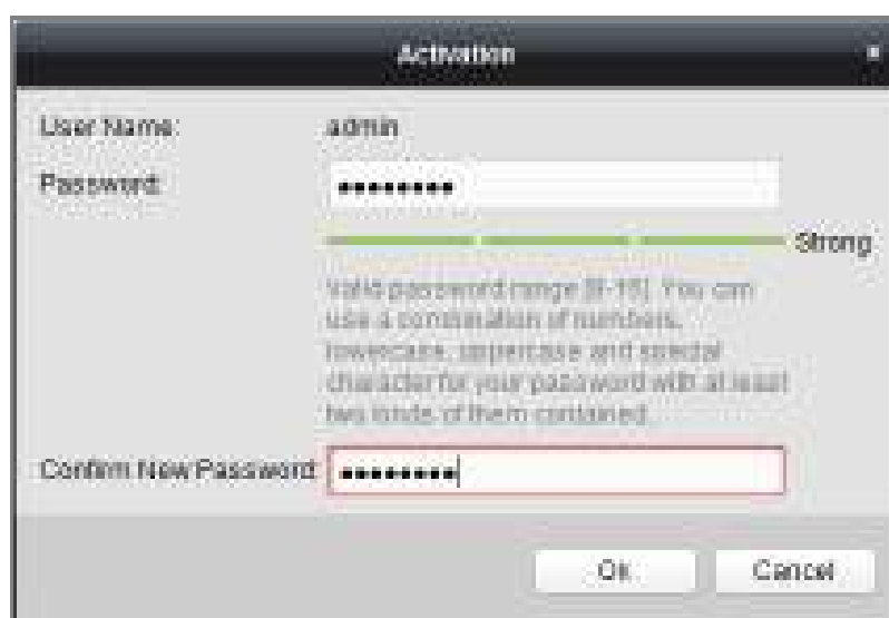
Figure 2-8 Activation Interface (Client Software)
