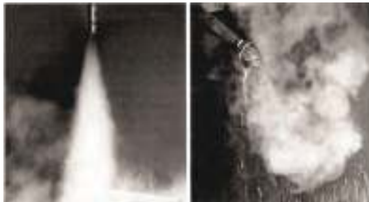
Figure 9.3.7. Live steam (left) versus flash steam (right)
