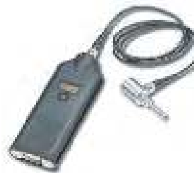
Examples of typical hand-held vibration sensing meters. Note readout providing immediate level indication.
