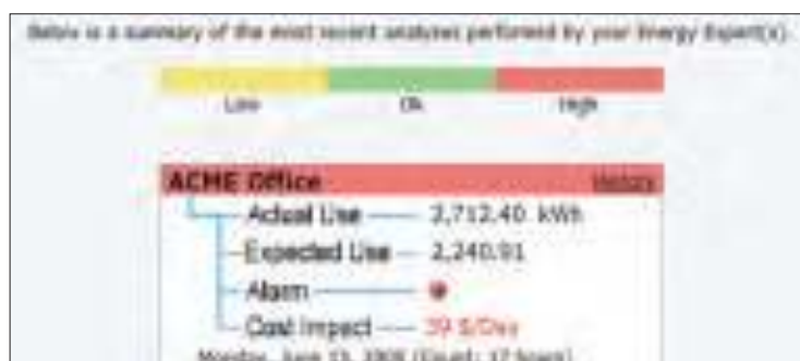
Figure 8.9.2. Sample screen capture for a generic building showing an alarm or high-energy using condition. Included is an estimated cost impact associated with the higher than expected electricity use.
