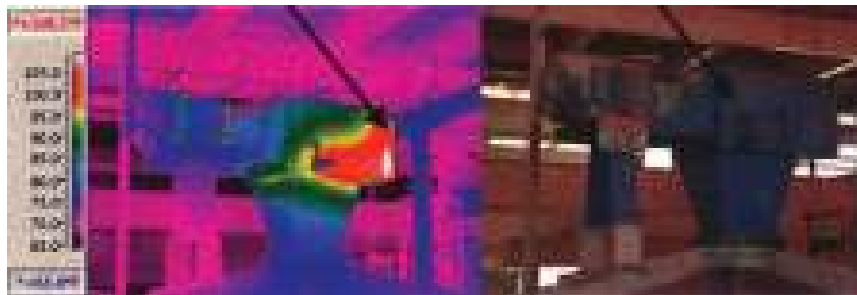
Figure 6.2.7. Possible gearbox problem indicated by white area defined by arrow. Design drawings of gearbox should be examined to define possible cause of elevated temperatures.
