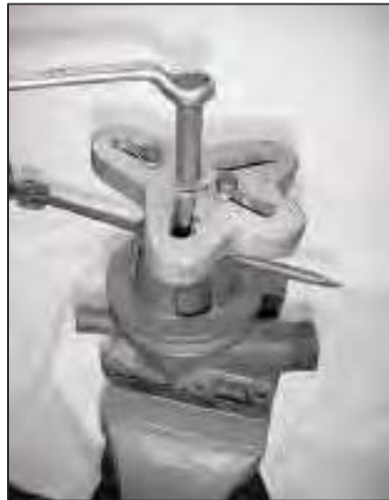
Fig. C2.34 Removal of Water Pump Pulley with SST #EF0300
