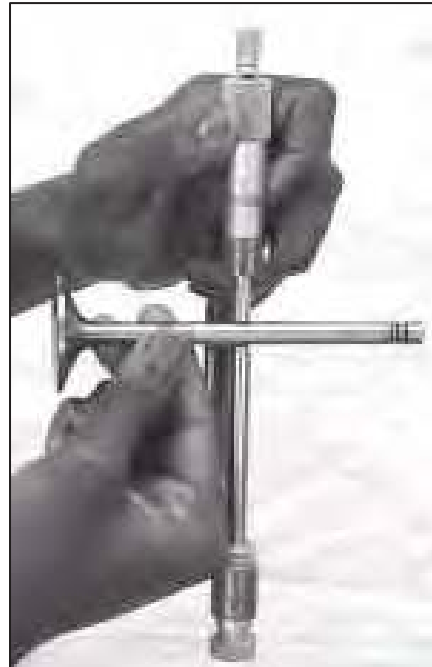
Fig. C2.40 Measuring the Valve Stem Diameter
