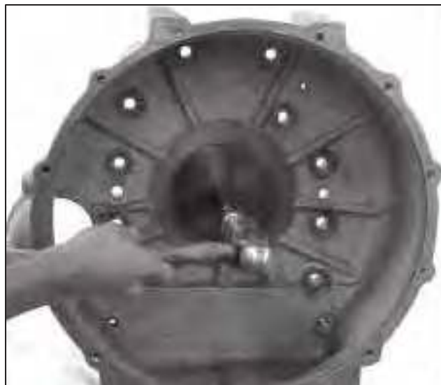
Fig. C2.28 Installing Rear Main Oil Seal
