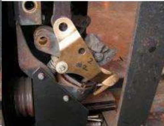
Figure 30. Hinge Pin and Spacers Removed
