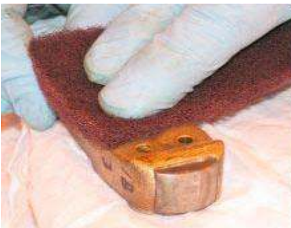
Figure 40. Buffing With Scotch Brite
