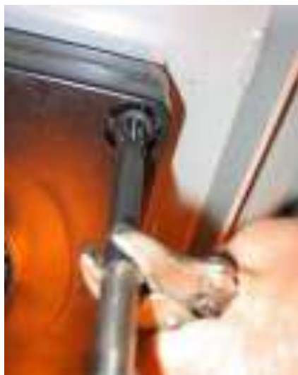
Figure 82. Reaming the Mounting Hole
