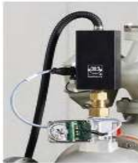
Figure 12. DensiControl IN Measuring Hose and Supplied Electrical Cable
