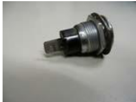
Figure 2. Receptacle Without a Resistor, Removed From the Mounting
