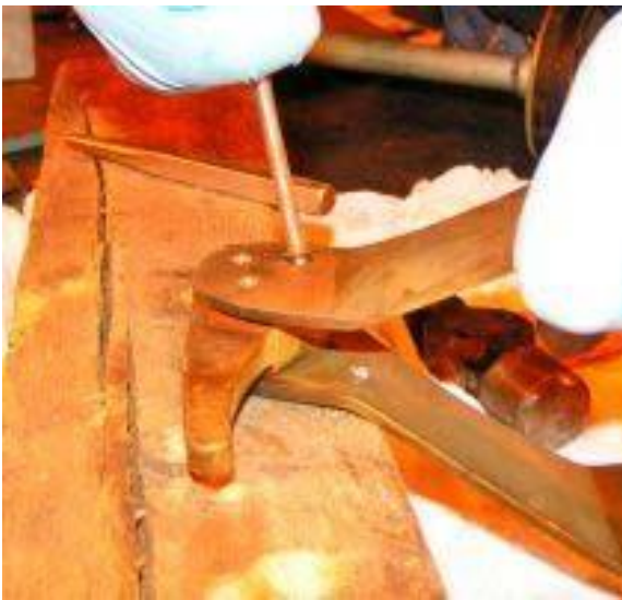
Figure 36. Breaking Off the Rivet Head
