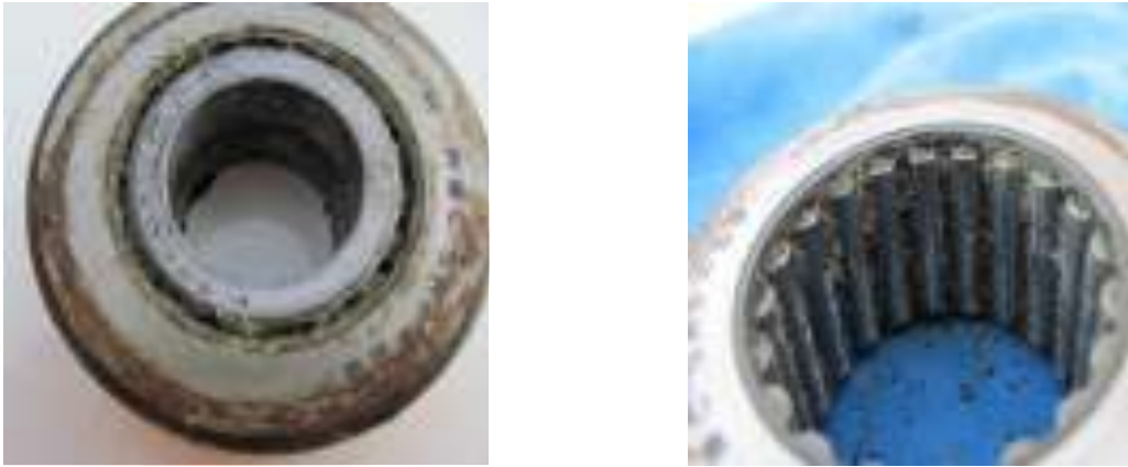
Figure 105. Trip Latch Bearing with Old, Hard Grease (External and Internal)
