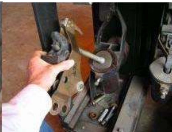
Figure 32. Lifting the Contact Assembly and Booster Piston
