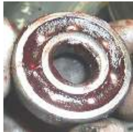
Figure 112. Fully Packed Open Ball Bearing
