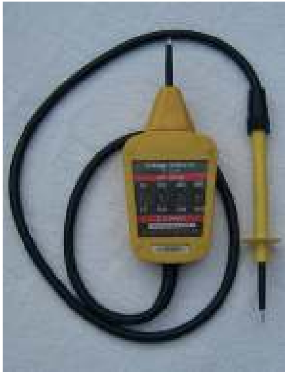
Figure 1.20 Typical voltage indicator.
