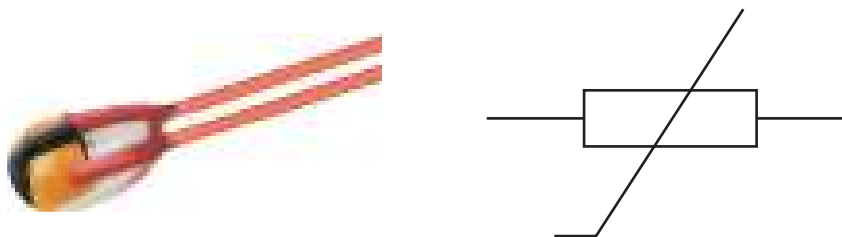
Figure 9.87 Symbol for and appearance of a thermistor.
