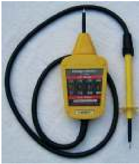
Figure 8.3 Typical voltage indicator.
