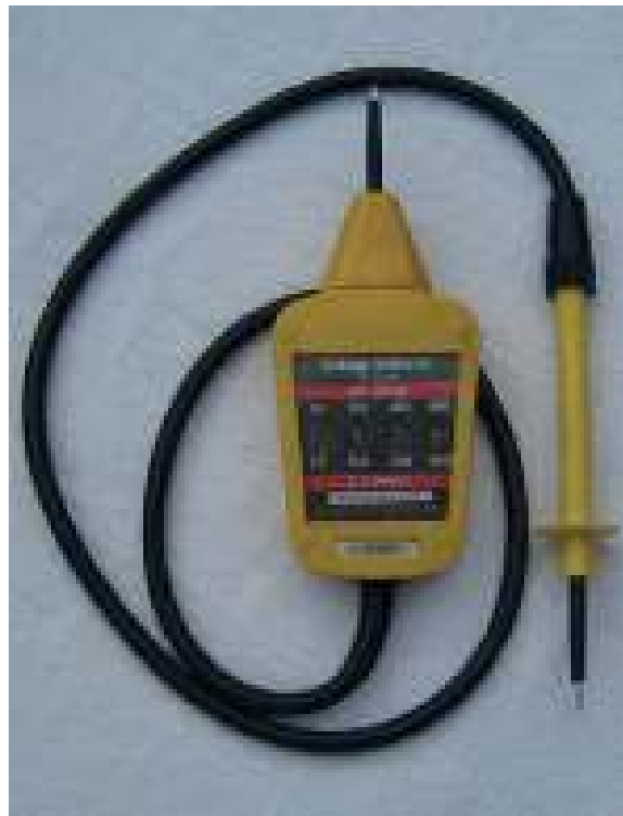
Figure 7.7 Typical voltage indicator.
