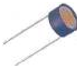
Figure 9.85 Symbol and appearance of an LDR.
