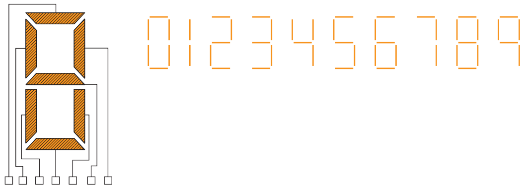
Figure 9.84 LED used in seven-segment display.
