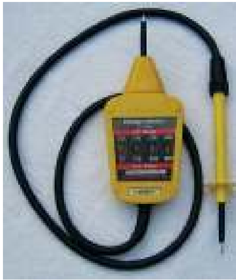
Figure 6.19 Typical voltage indicator.
