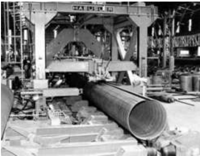
Figure 11.14 Pipe welding machine.
