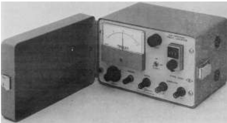
FIGURE 5.42 Portable Murray loop resistance bridge for cable fault-locating work. (Courtesy of James G. Biddle Company.)
