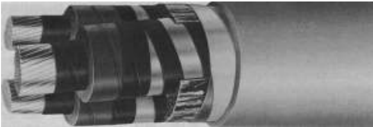
FIGURE 5.3 Three-conductor shielded (tape-H), compact sector, paper-insulated cable. (Okonite Bulletin PCI-1979; copyright 1979.)
