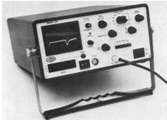
FIGURE 5.45 Automatic digital radar cable test set. (Courtesy of James G. Biddle Company.)
