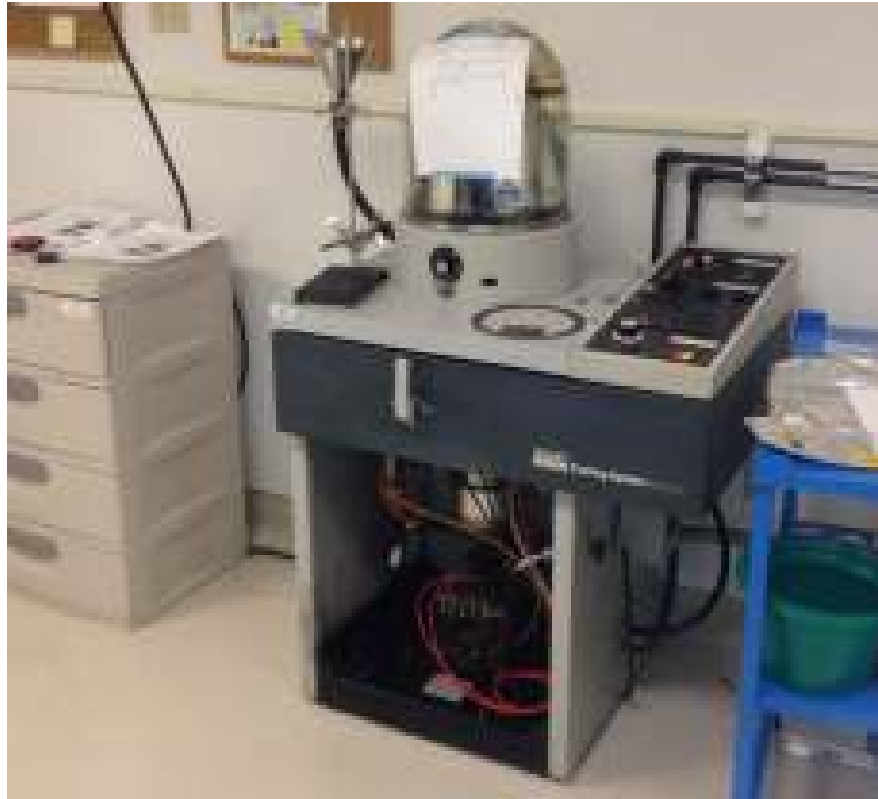
Fig. 5.3.1.a – This thermal evaporator was placed out of service because of a fluid leak. Although the power switch was turned off and the control panel showed no visible sign of electric power, the cord was still plugged in (behind the drawer cabinet to the left) and the 220V transformer in the bottom (next to the red wires) had exposed live parts. The cover panel, which was removed, did not have any shock hazard warning label. The evaporator is not listed by an NRTL and had not been inspected under the Electrical Equipment Safety Program. The evaporator should have been inspected, labeled, and unplugged prior to removing the panel.
