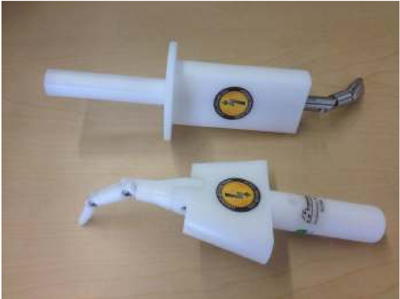
Fig. 7.2.3 – Articulated Test Fingers. IEC at the top, UL at the bottom.
