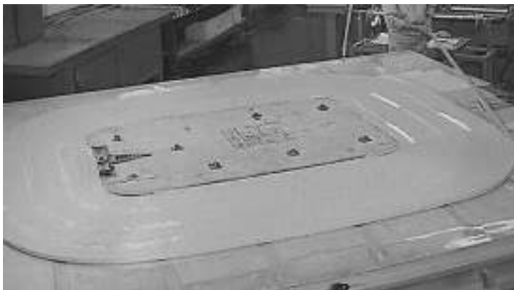
FIGURE 2.12 Pancake winding during winding process.
