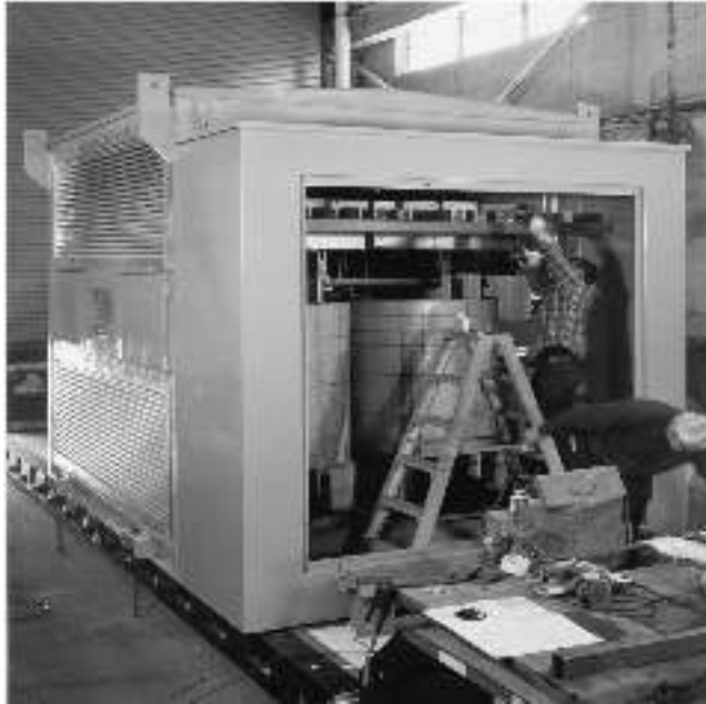
FIGURE 5.20 A 24-pulse dry-type transformer. 7000-kVA drive duty transformer, to be located in a tunnel, made of two 3500-kVA 12-pulse transformers. Each core and coil has 1100-V delta and wye secondary windings. Each core and coil has a 13,200-V extended-delta primary winding. One core and coil has its primary winding shifted -15^\circ , while the other core and coil has its primary winding shifted +15^\circ . One reconnectable primary spare core and coil can be used to replace either core and coil assembly. (Photo courtesy of Niagara Transformer Corp.)
