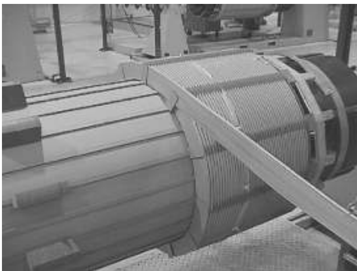
FIGURE 2.15 Helical winding during assembly.
