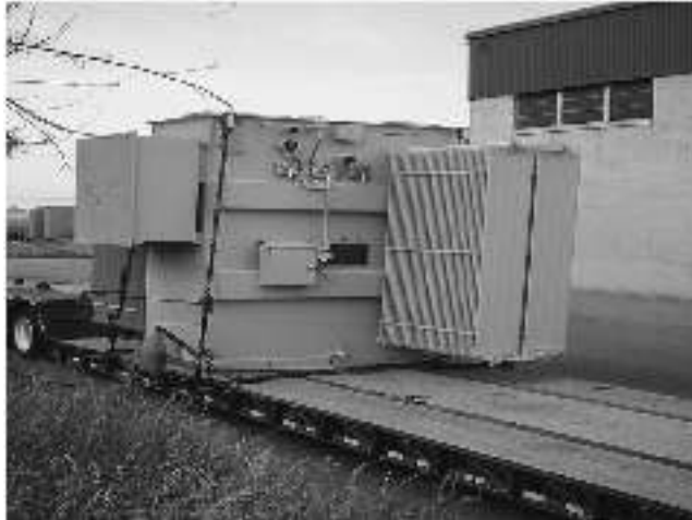
FIGURE 5.22 A 5000-kVA 18-pulse transformer ready for shipment. Motor drive duty, 13,800-V delta primary to secondaries of 1400-V delta, 1400-V delta +20^\circ , and 1400-V delta -20^\circ . (Photo courtesy of Niagara Transformer Corp.)
