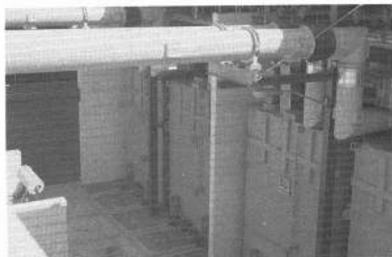
Figure 8.7 Test transformers installed at the LAPEM laboratory. Two transformers per phase are used in this installation. (Courtesy of LAPEM, Irapuato, Gto., Mexico.)
