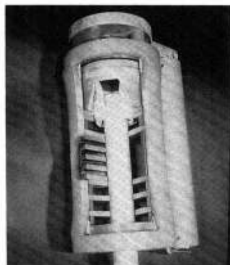
Figure 5.23 Oil breaker interrupting chamber showing lateral vents.
