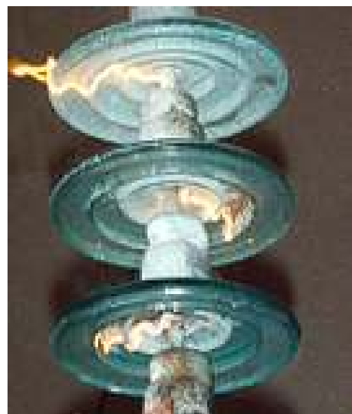
Fig. 3.34: Polluted Glass Cap and Pin Insulator string with dry bands
