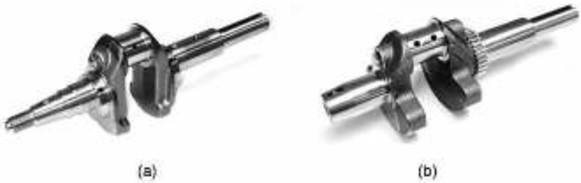
FIG. 7-37 Forged (a) and cast-iron (b) crankshafts used in Dr. Fatemi's study.
