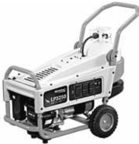
FIG. 1-5 A Generac residential generator, rated at 3250 W and adapted for propane use. The 20-lb tank provides 9 hours of half-load running time between refills. Gempeler's
