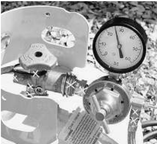
FIG. 2-9 Using soapy water, check the X-ed joints for leaks. City of New York Fire Department
