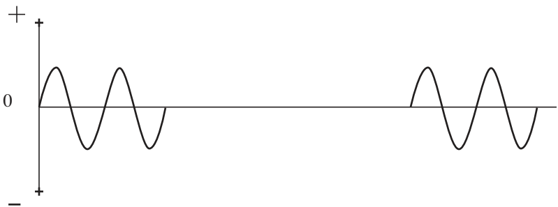
FIG. 4-2 Output from a two-coil flywheel alternator. Output goes flat until the magnets again swing into position adjacent to the coils. Multiple-coil alternators have much smoother outputs.
