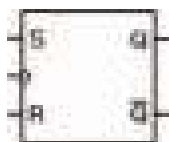
Figure 11.13 A clocked, edge-triggered, SR-type bistable symbol
