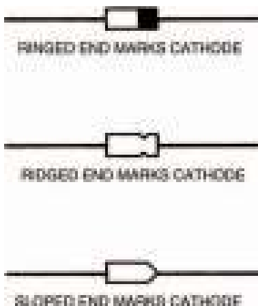
Figure 6.2 Some typical diode body shapes
