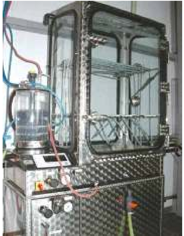
Environmental ageing chamber for ammonia atmosphere ageing
