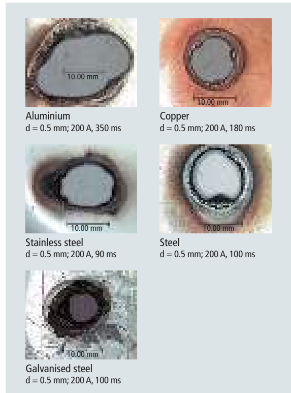
Figure 2.4.3 Plates perforated by the effects of long stroke arcs
