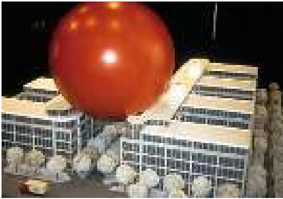
Figure 5.1.1.4 New administration building: Model with rolling sphere according to class of LPS I; source: WBG Wiesinger
