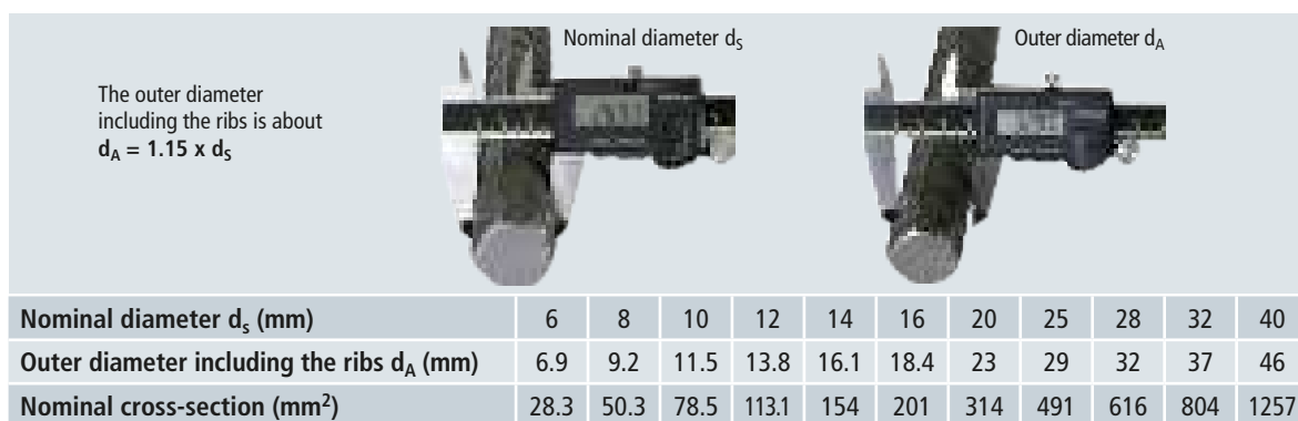
Figure 5.5.2.7 Diameters of reinforcing steels
