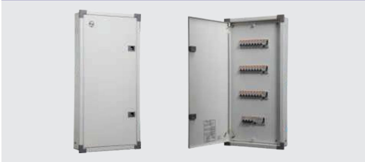
Metal Tier DBs for Three-Phase and Neutral (TPN ) supply distribution with Per Phase Isolation (PPI)
