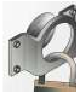
Obstruction of the lever hub socket by padlock
