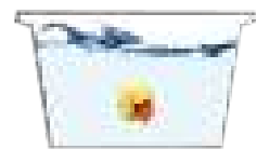
IP67: Submersion to one meter for 30 minutes.
