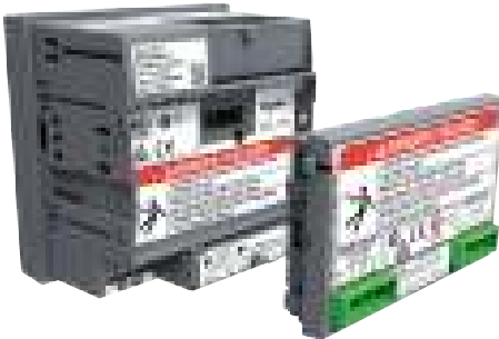
Rear of PM2000 with I/O module disconnected
