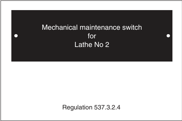
Figure 9.11 Mechanical switch notice
