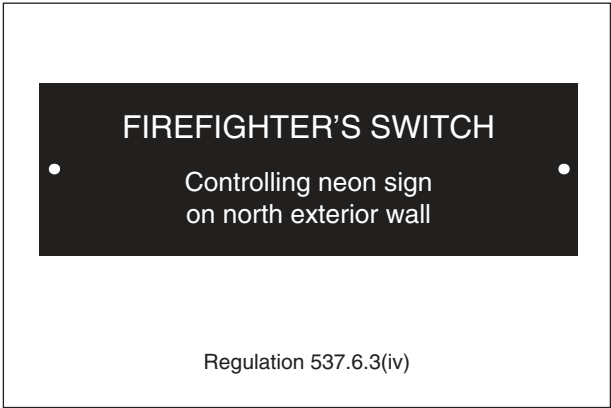
Figure 9.20 Remote fireman's switch notice
