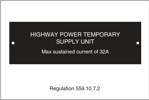
Figure 9.22 Highway power temporary supply unit notice
