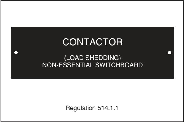
Figure 9.16 Contactor designation notice
