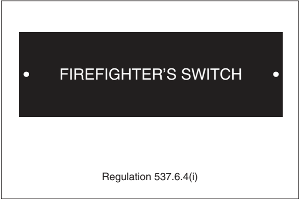
Figure 9.19 Firefighter’s switch notice
