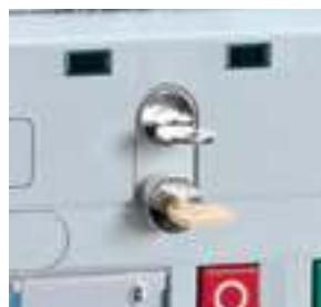
^ Key locking in open position
