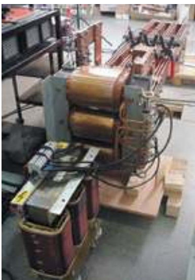
< Temperature rise test for a 3 x 120 x 10 per pole busbar on support Cat. No. 374 54
