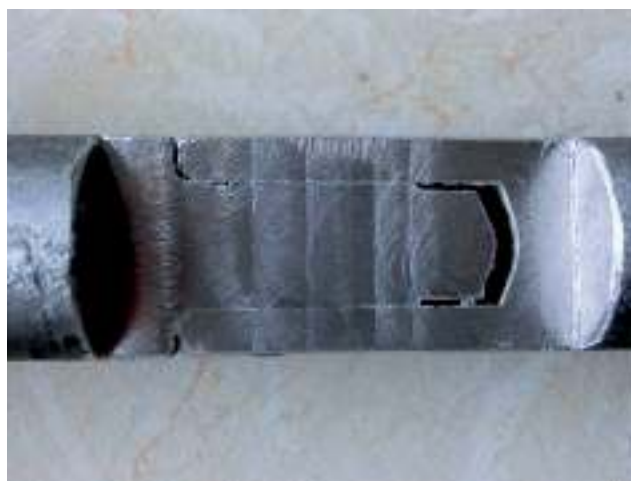
Cross-section through the coupling of an OBO earth rod
