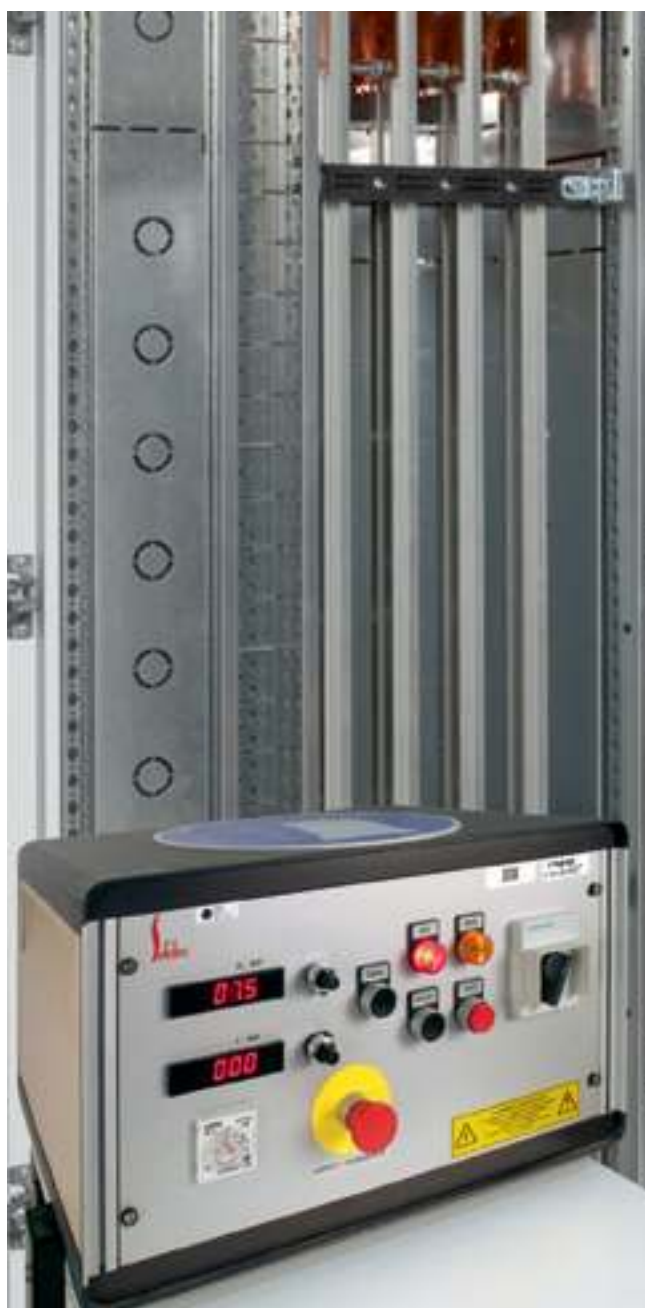
Industrial frequency > generator for insulation test
