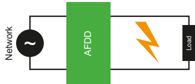
Fig. F81 Parallel arc fault
