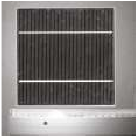
Fig. P3 Photovoltaic cell manufactured in a silicon plate (source: Photowatt)
