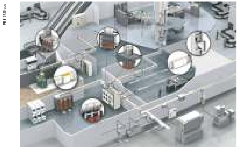
Fig. E45 Radial distribution using busways
