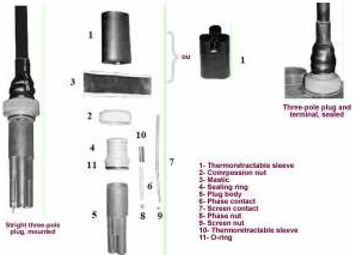
Figure 141: Right three-pole plug and terminal, 6kV
