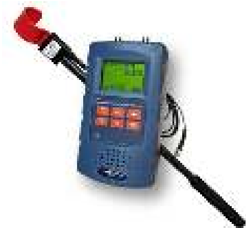
Figure 232: Detector of partial discharges - ultrasounds
