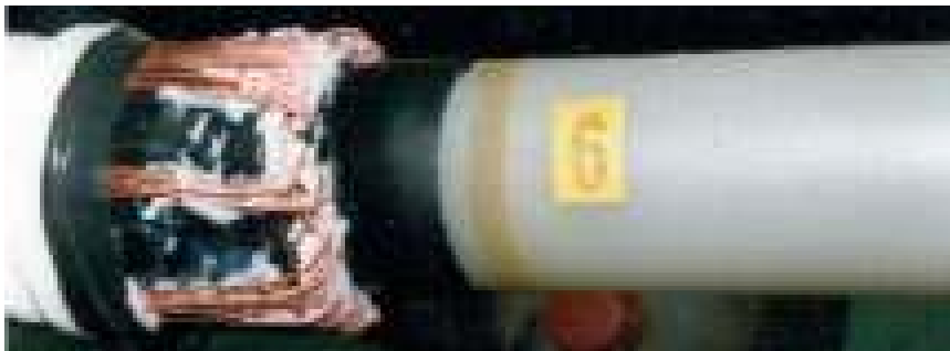
Figure 150: Fault on single-pole 24kV cable
