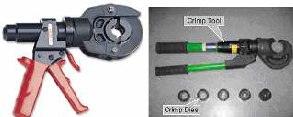
Figure 179: Hydraulic hand operated crimping tool
