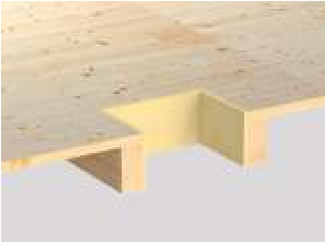
Wooden beam ceiling without fire protection ceiling
