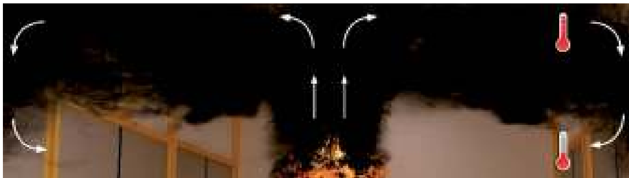
Heat build-up under the ceiling in the event of a fire
