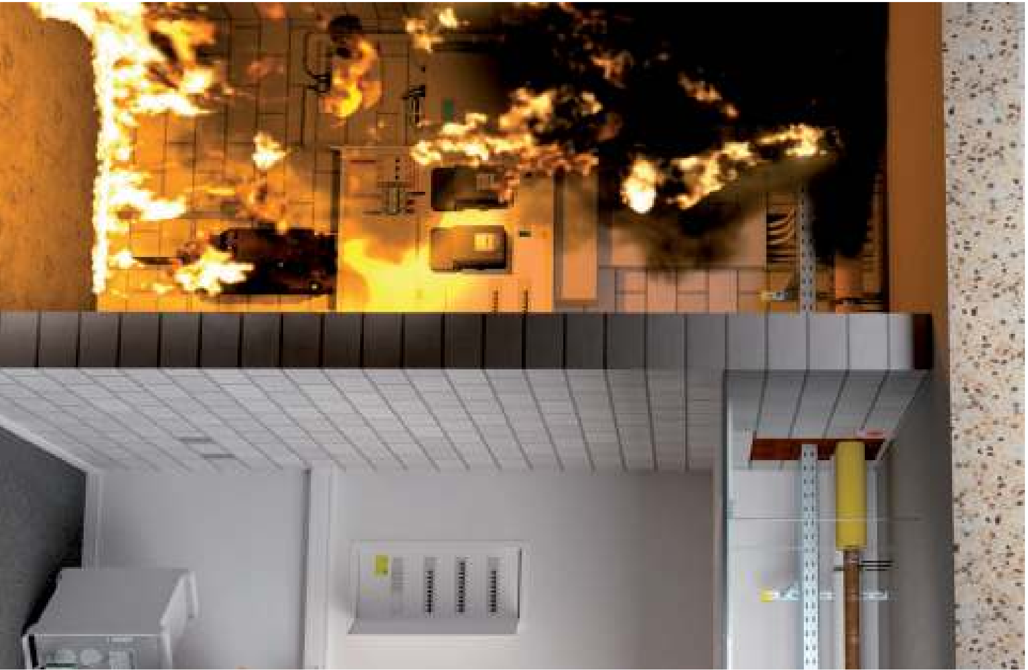
Ceiling and wall penetrations can be sealed reliably against fire and smoke
