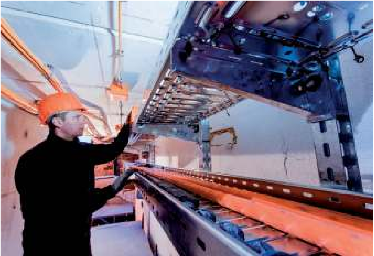
Test structure of a cable system that maintains electrical functionality
