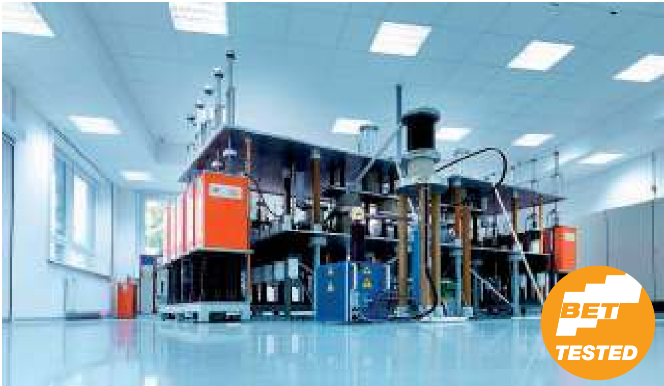
BET lightning current generator and BET test mark
