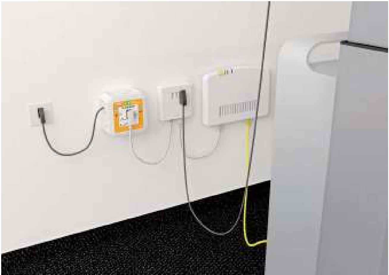
Protection of an ISDN + DSL connection with TeleDefender
