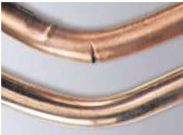
Figure 76. Copper bonded and copper clad earth rods.
