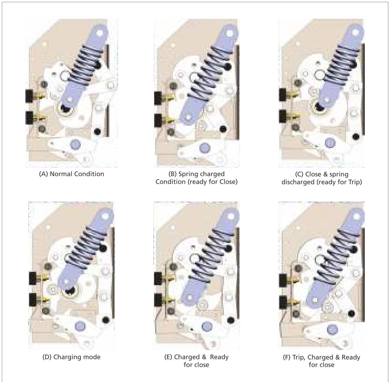
Figure 13 : Motor stored energy mechanism
