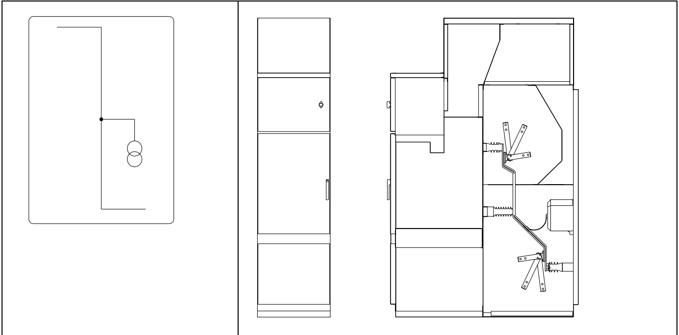
Busbar riser with fixed measuring VT
