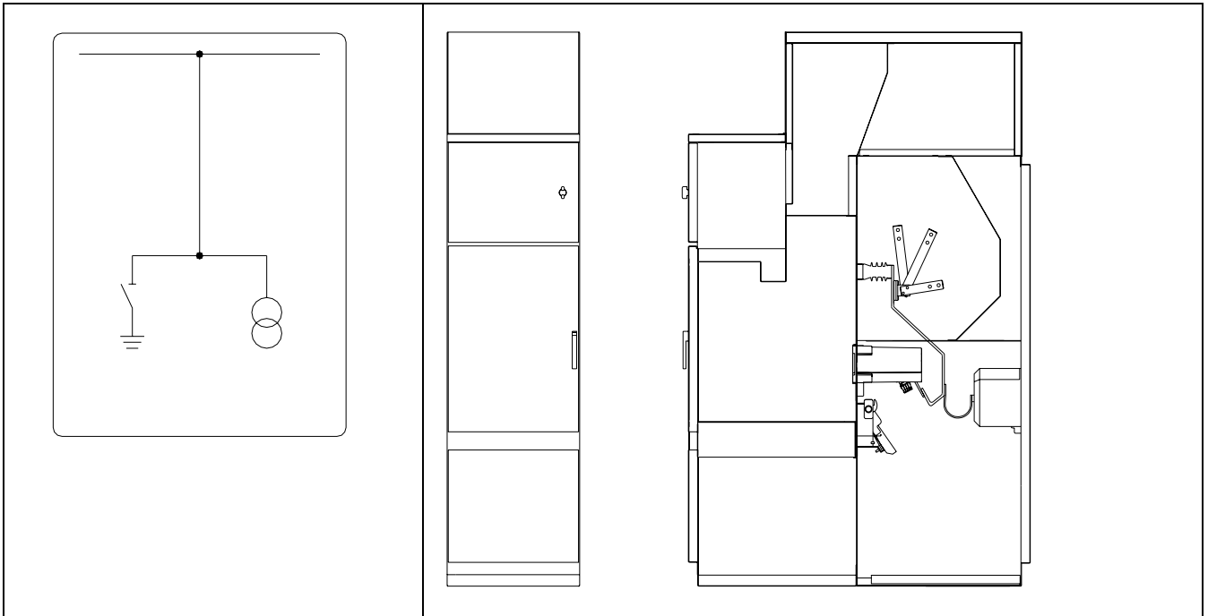
Measurement panel with Fixed VT and earthing switch.
