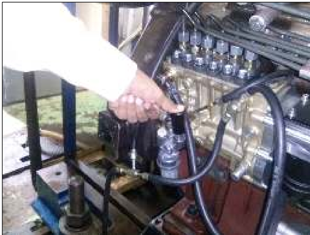
Fig. C3.17 Illustration of Air Removal from Fuel System
