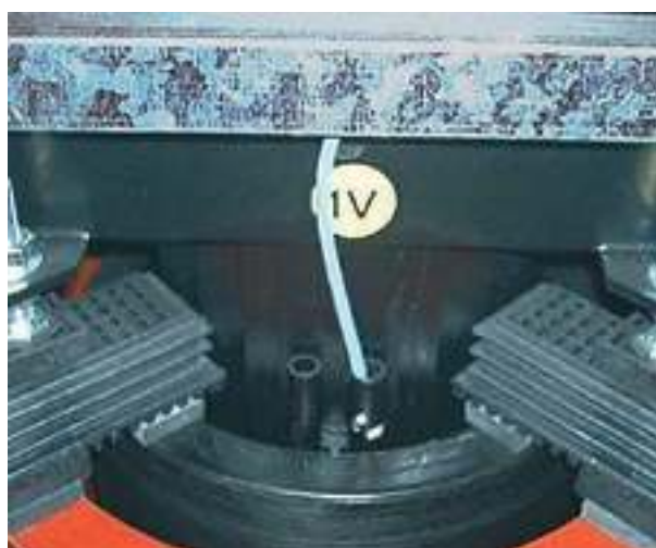
^ PCT sensor to check the temperature
