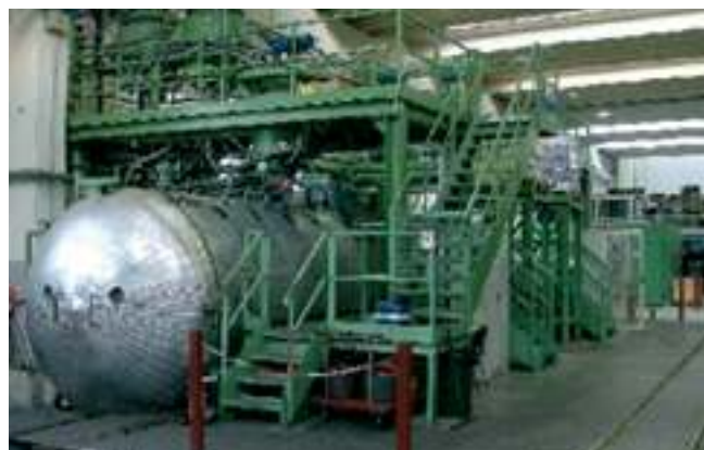
^ The pouring system under high vacuum
