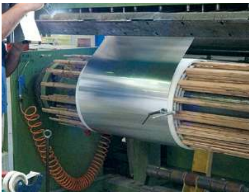
< TIG welding in controlled atmosphere for LV connections.
