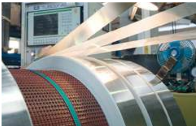
^ Modern electronically controlled winding machines
