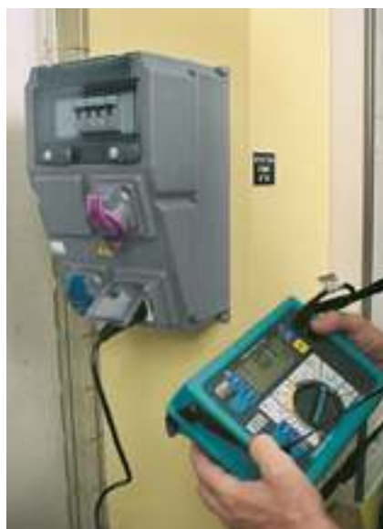
< On-site measurement of the end of line short-circuit value provides practical validation of the choice of protection
