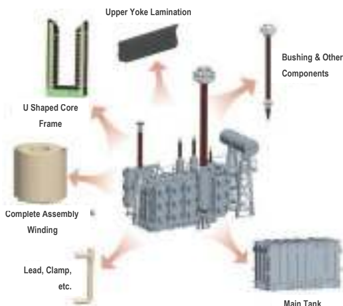
(a) Assembled transformer after factory tests (b) Diagram of disassembly of each component
