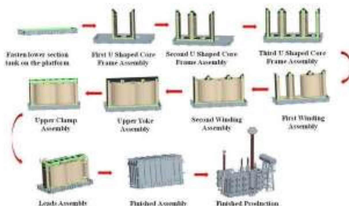
Figure 2.42 - Assembly process flow inside field assembly building
