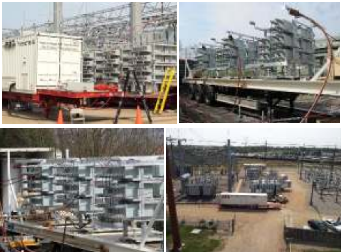
Figure 4.9 - Additional external capacitive compensation for temperature-rise tests
