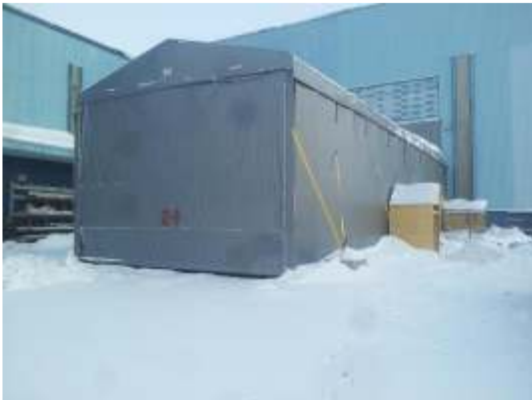
Figure 4.28 - Temporary housing for the test system - protection from the weather condition
