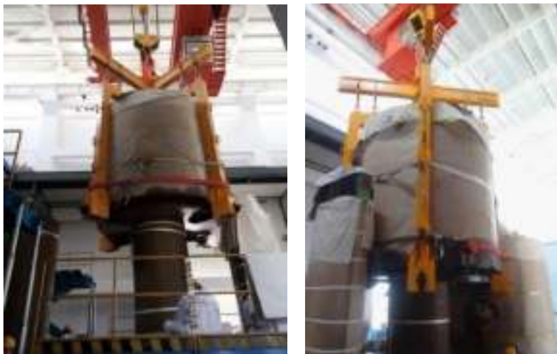
Figure 2.45 - Assembly of winding columns and its end product
