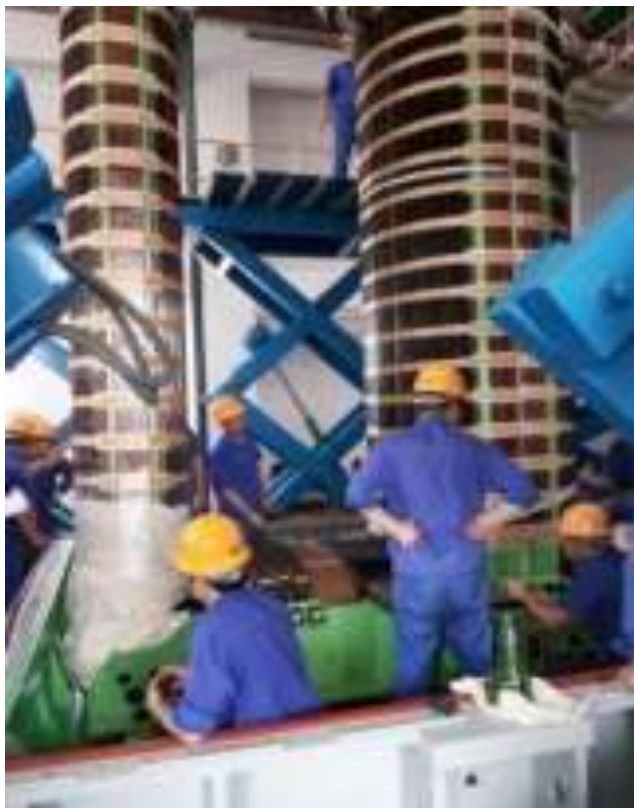
Figure 2.44 - Assembly of U-shaped core frames and its end product
