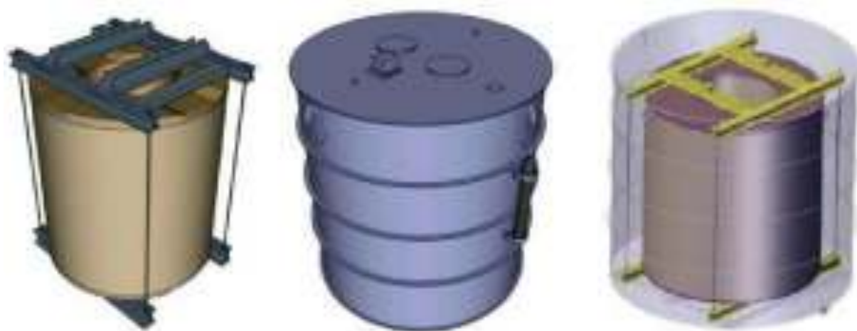
Figure 2.39 - Single transportation unit for winding column
