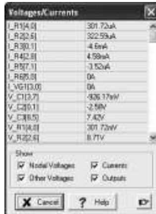
Figure 12.8: Results of DC analysis of circuit shown in Fig. 12.6
