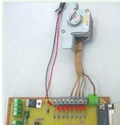
Connecting a stepper motor to the interface
