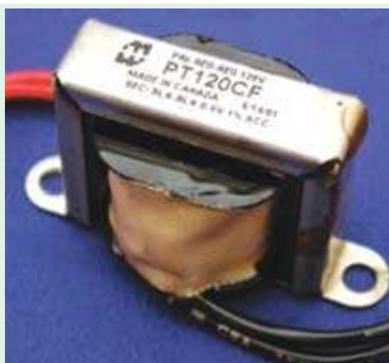
Small Potential transformer
