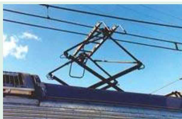
The pantograph mechanism helps to maintain a link between the overhead contact wire and power circuit of the electric locomotive
