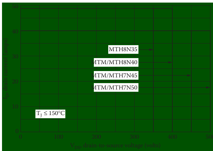
Figure 6.6 Maximum rated switching safe operating area of the MTM8N40 MOSFET. (Courtesy of Motorola.)
