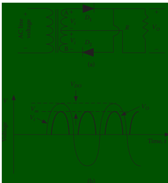
Figure 7.7 Full-wave rectifier circuit: (a) schematic diagram, (b) input and output waveforms. (From [2]. Used with permission.)
