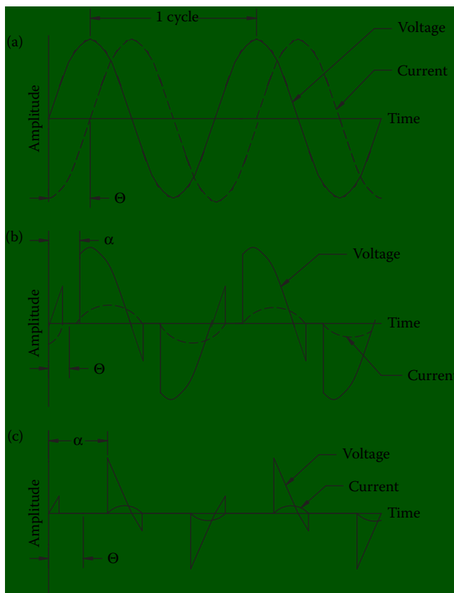
Figure 8.5 Voltage and current waveforms for inverse-parallel thyristor power control with an inductive load: (a) full conduction; (b) small-angle phase reduction; (c) large-angle phase reduction.
