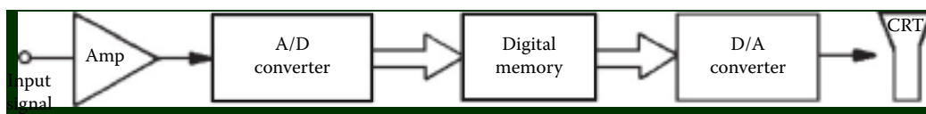
Figure 10.11 Simplified block diagram of a digital storage oscilloscope.
