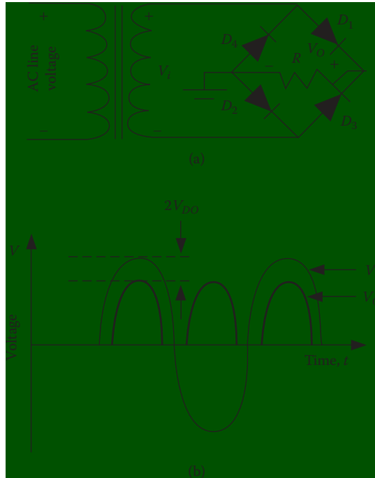
Figure 7.8 Bridge rectifier circuit: (a) schematic diagram, (b) input and output waveforms. (From [2]. Used with permission.)
