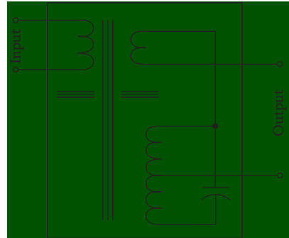
Figure 14.1 Basic design of a ferroresonant transformer. (After [1].)
