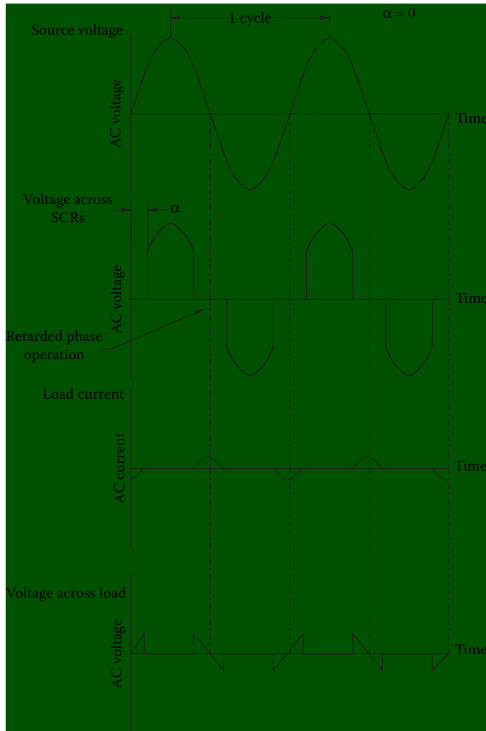
Figure 8.4 Waveforms in an ac circuit using thyristor power control.
