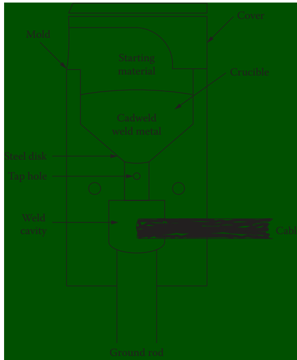
Figure 18.21 Typical exothermic bonding mold for connecting a cable to a ground rod. (After [9].)
