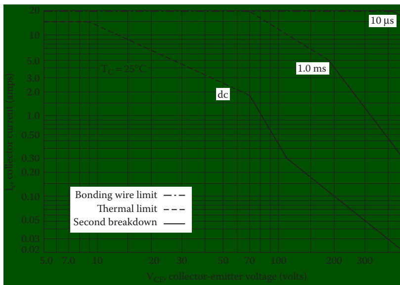
Figure 6.1 Forward bias safe operating area curve for a bipolar transistor (MJH16010A). (Courtesy of Motorola.)
