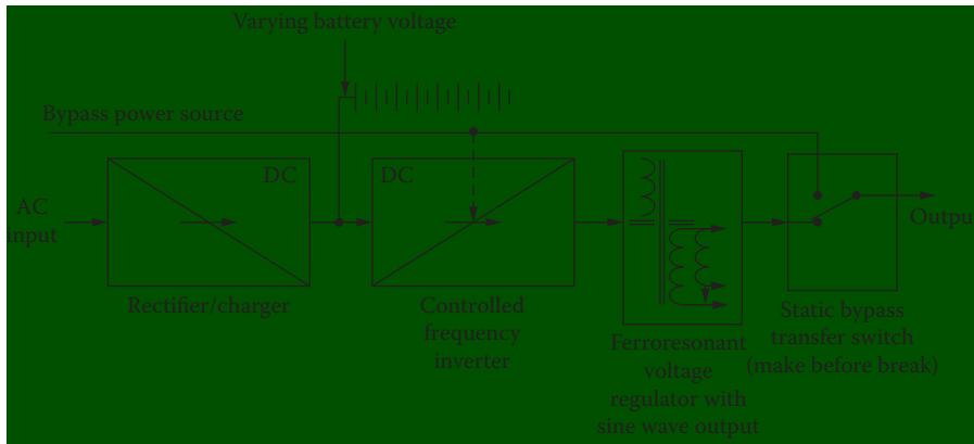
Figure 13.7 Simplified diagram of a static UPS system based on a ferroresonant transformer. (After [1]).
