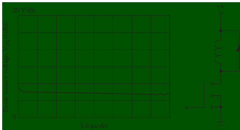
Figure 6.8 Drain-source transient with a clamping diode across the inductive load. (Courtesy of Motorola.)
