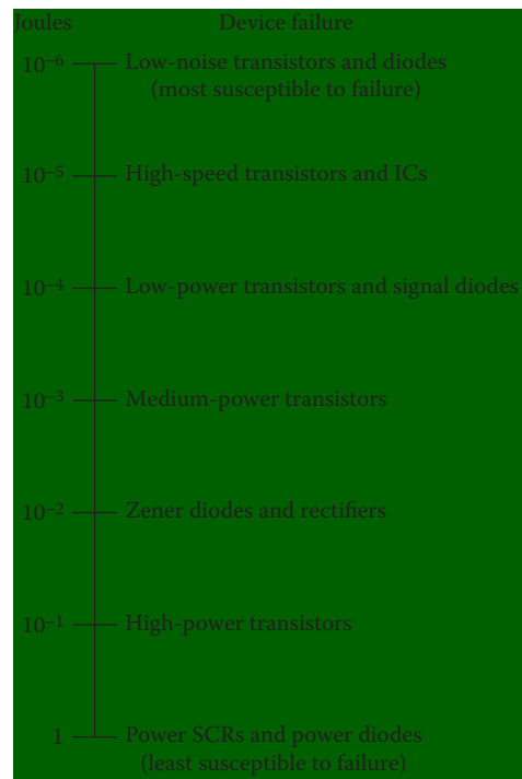
Figure 6.16 An estimate of the susceptibility of semiconductor devices to failure because of transient energy. The estimate assumes a transient duration of several microseconds.
