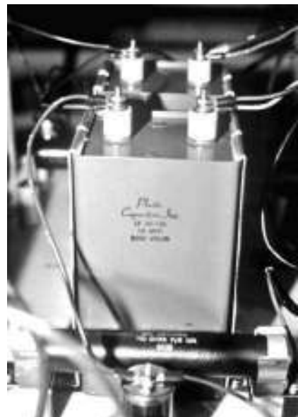
Figure 5.5 An oil-filled, high-voltage capacitor.
