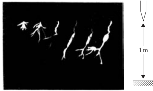
Figure 1.10 Streak photograph of development of a negative leader system, showing negative streamers ahead of the leader tip and retrograde streamers towards the anode [20]
