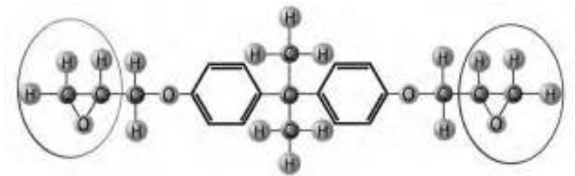
Figure 8.9 Chemical composition of basic epoxy resin. Epoxide functional groups are circled. These groups are characteristic for every epoxy, but the polymer chain in between them can vary
