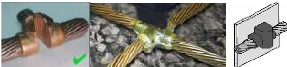
Figure 19: Examples of good weld joints with aluminothermic method
