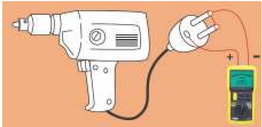
Figure 62: Insulation measurements on electrical equipment
