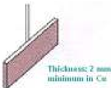
Figure 8: Earth Electrode in vertical plate
