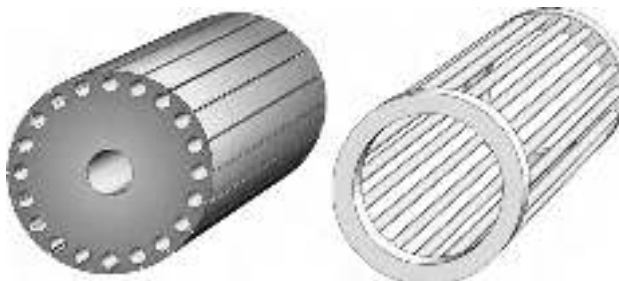
Figure 5.10 Cage rotor construction. The stack of pre-punched laminations is shown on the left, with the copper or aluminum rotor bars and end-rings on the right.
