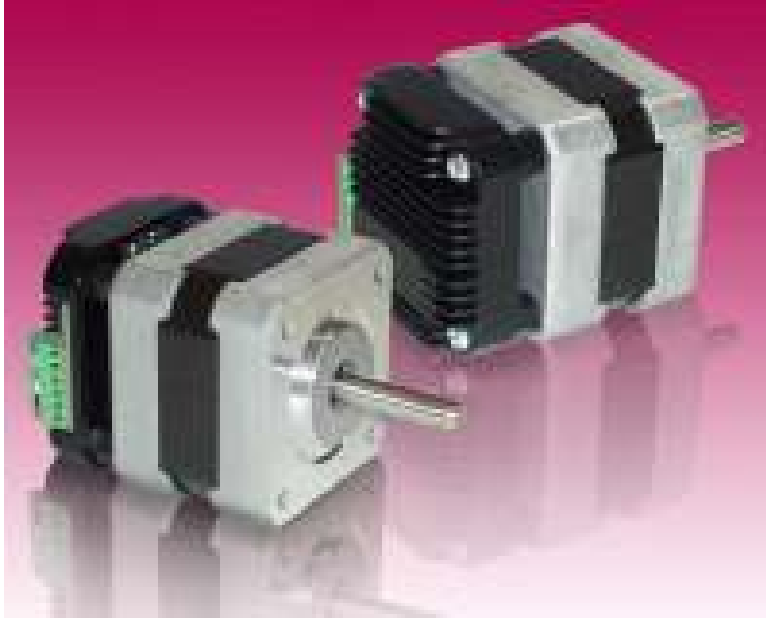
Plate 10.5 The die-cast aluminum construction of these self-contained mini-stepping bipolar drivers provides efficient heat dissipation, and they are designed for retrofitting to existing size 17 motors. (Courtesy of Astrosyn)
