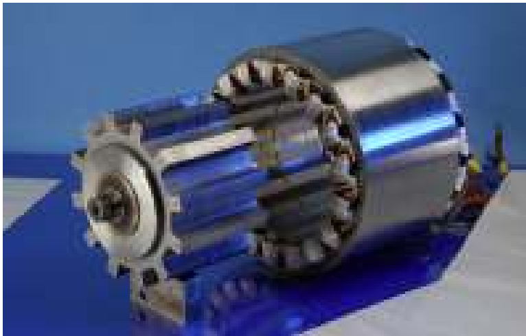
Plate 10.6 Switched Reluctance Motor. The toothed rotor does not require windings or magnets, and is therefore exceptionally robust. (Courtesy of Nidec S R Drives Ltd.)
