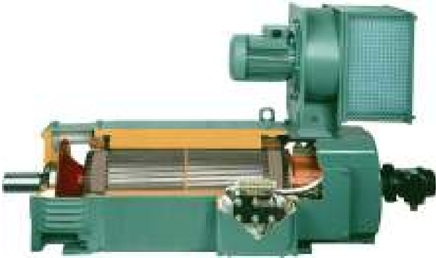
Plate 4.1 High performance force-ventilated d.c. motor. The motor is of all-laminated construction and designed for use with a thyristor converter. The small blower motor is an induction machine that runs continuously, thereby allowing the main motor to maintain full torque at low speed without overheating. (Courtesy of Emerson – Leroy Somer)
