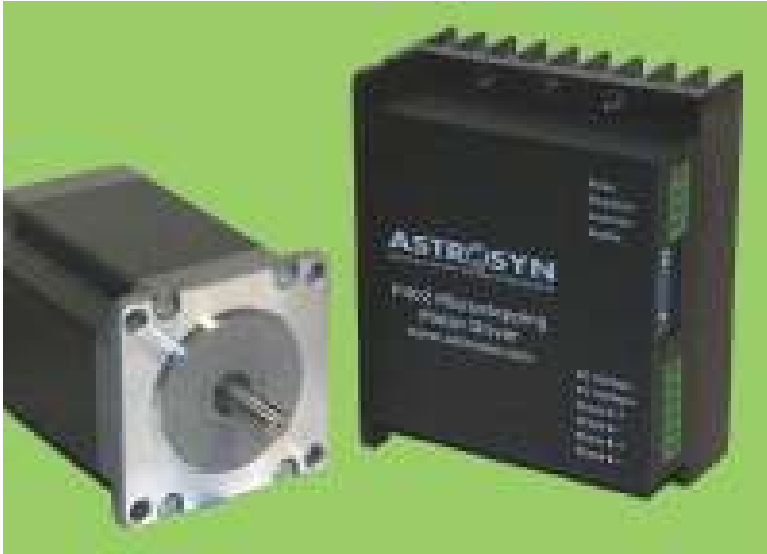
Plate 10.3 This bipolar chopper mini-stepping drive with integral heatsink provides a range of step divisions up to 25,600 steps/rev and allows drive current to be set from 0.25 A to 2.0 A with supply voltage from 14 V to 40 V. (Courtesy of Astrosyn)
