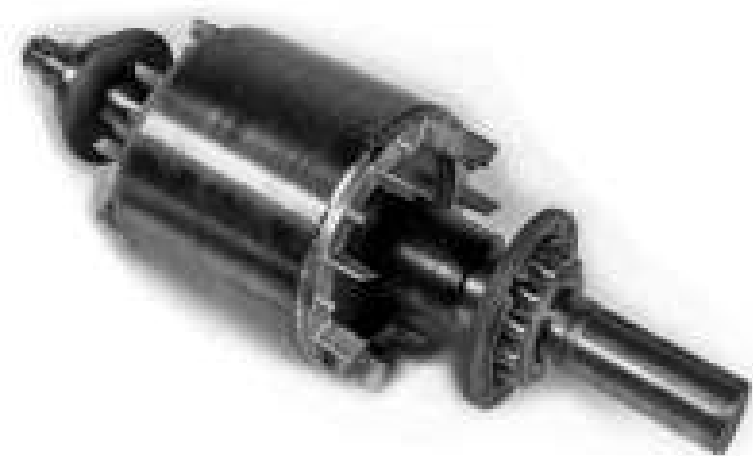
Plate 5.2 Cage rotor for induction motor. The rotor conductor bars and end rings are cast in aluminum, and the blades attached to the end rings serve as a fan for circulating internal air. An external fan will be mounted on the non-drive end to cool the finned stator casing (as shown in Figure 8.4). (Courtesy of Brook Crompton)
