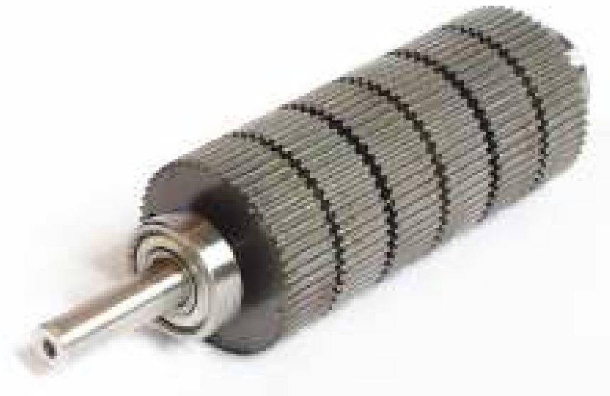
Plate 10.2 Rotor of size 34 (3.4 inch or 8 cm diameter) 3-stack hybrid 1.8° stepping motor. The dimensions of the rotor end-caps and the associated axially-magnetized permanent magnet are optimized for the single-stack version. Extra torque is obtained by adding a second or third stack, the stator simply being stretched to accommodate the longer rotor. (Courtesy of Astrosyn)
