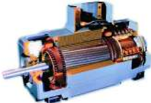
Plate 3.1 Cutaway view of 4-pole d.c. motor. The skewed armature windings on the rotor are connected at the right-hand-end via risers to the commutator segments. There are four sets of brushes, and each brush arm holds four brush-boxes. The sectioned coils surrounding two of the four poles are visible close to the left-hand armature end-windings. (Courtesy of ABB)
