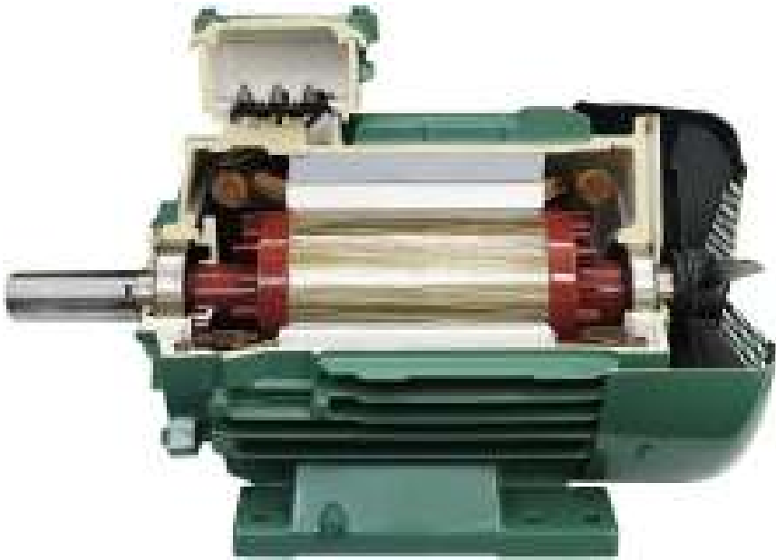
Plate 8.4 Typical shaft-mounted external cooling fan on an a.c. induction motor. (Courtesy of Emerson – Leroy Somer)
