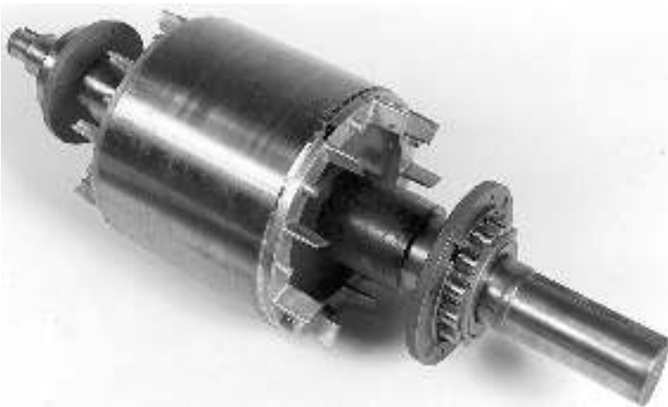
Plate 5.2 Cage rotor for induction motor. The rotor conductor bars and end rings are cast in aluminium, and the blades attached to the end rings serve as a fan for circulating
