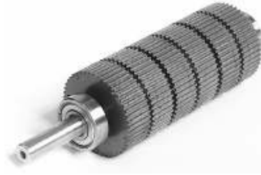
Plate 9.2 Rotor of size 34 (3.4 inch or 8 cm diameter) 3-stack hybrid 1.8° stepping motor. The dimensions of the rotor end-caps and the associated axially-magnetised permanent magnet are optimised for the single-stack version. Extra torque is obtained by adding a second or third stack, the stator simply being stretched to accommodate the longer rotor. (Photo by courtesy of Astrosyn)
