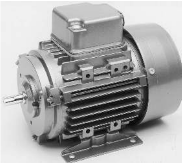
Plate 1.1 Totally enclosed fan-ventilated (TEFV) cage induction motor. This particular example is rated at 200 W (0.27 h.p.) at 1450 rev/min, and is at the lower end of the power range for 3-phase versions. The case is of cast aluminium, with cooling air provided by the covered fan at the non-drive end. Note the provision for alternative mounting. (Photograph by courtesy of Brook Crompton)
